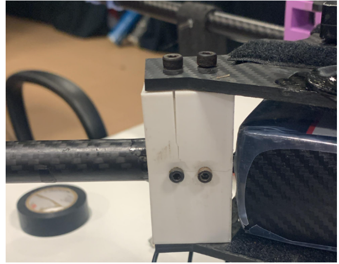
Figure 9: Damaged PLA parts
