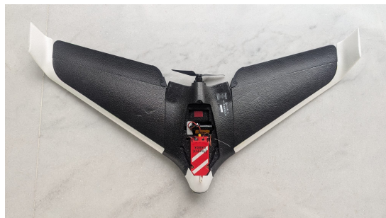
(a) Parrot Disco with onboard computer vision, flown with Paparazzi-UAV software [3] The cover is removed to show the c.h.u.n.c.k. computer-vision enabled autopilot. The autopilot has a front and bottom camera.
