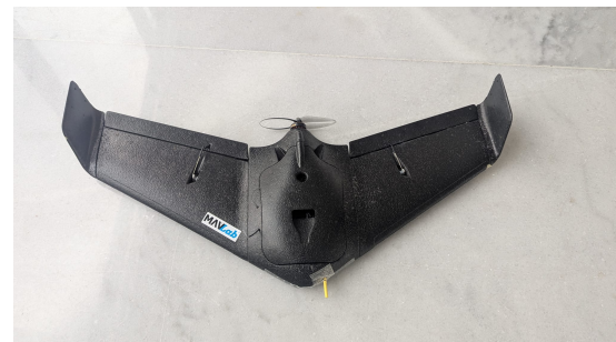
(b) 'Baby AR Wing Pro' airframe fitted with a Paparazzi-UAV Lisa-MX autopilot, Ublox GPS, a pitot tube and sensor, an remote magnetometer in the tip, a downward ranger for landing and modems.
