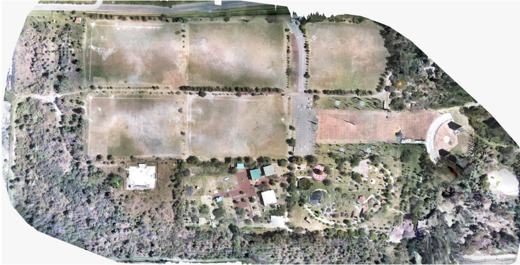
Figure 9: Mission 1: GPS-referenced Orthophoto reconstruction of the flight area during the competition slot. The map was generated by merging \sim 1300 downward-looking 320 \times 240 images from the Disco bottom camera using Open Drone Map [4].
