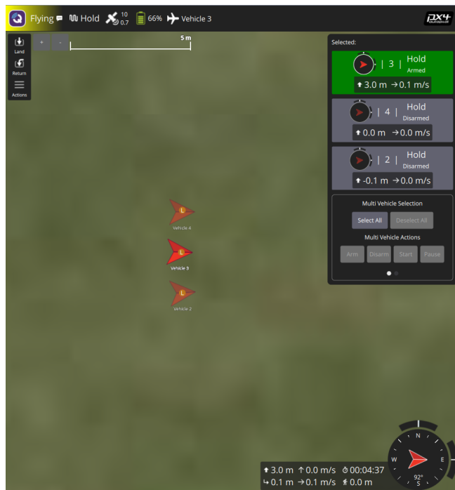
Figure 5: Swarm setup in QGroundControl system.
