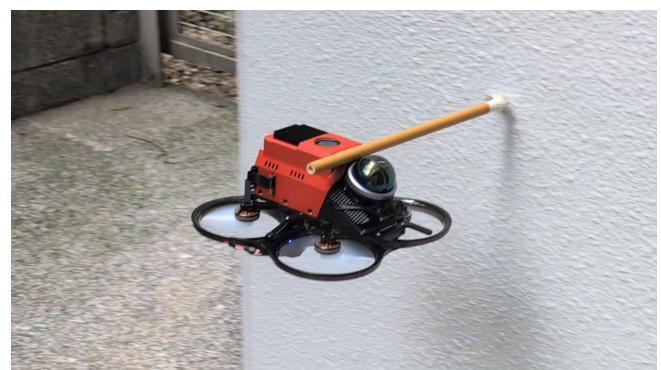
Figure 3: Chinese paint brush as the chosen writing tool. The figure shows the MAV emulating drawing on the wall using the paint brush. The paint brush can maintain good contact with the wall despite lateral position variations.
