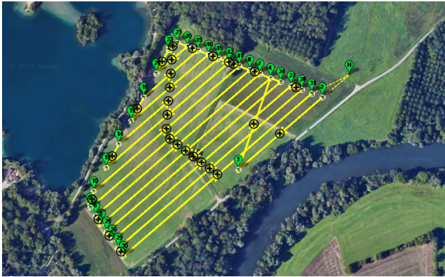
Figure 7: Grid used for a mapping with L_{line} = 16m
