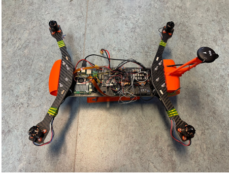
Figure 5: Integration of the Pixhawk, PM07 and Raspberry Pi.
