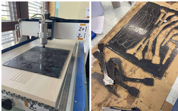
Figure 2: Left: CNC machining process. Right: Example of a finished drone part.
