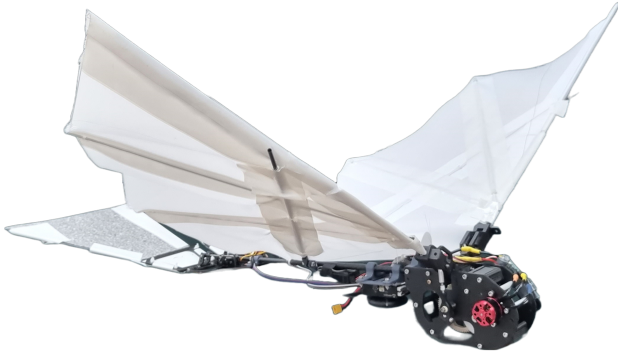
Figure 9: Fabricated flapping-wing air vehicle
