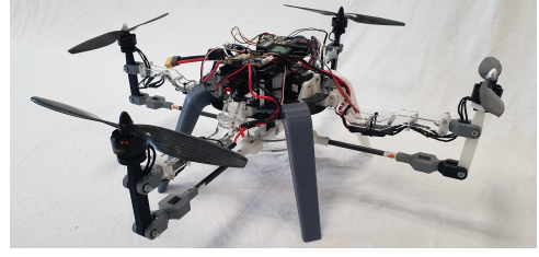
Figure 3: The prototype variable-tilt UAV developed for validation
