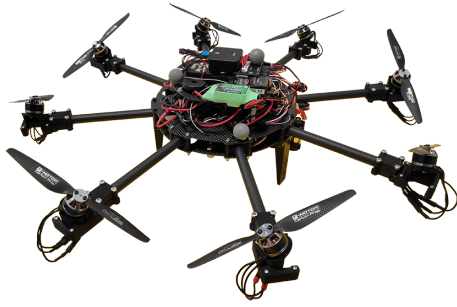
Figure 2: Photo of the canted-rotor planar octorotor UAV
