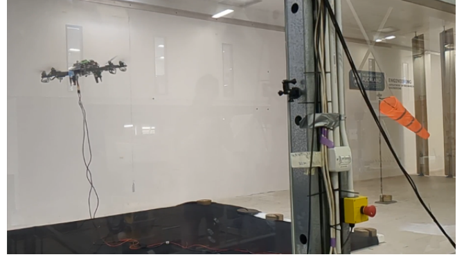
Figure 5: CRPO station-keeping in the BLWT under surging flow. Wind sock visually indicates wind direction.
