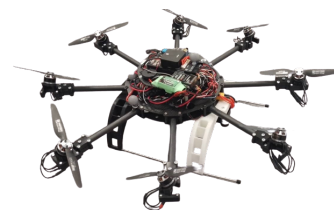
Figure 1: Fixed-tilt Octocopter, utilised in [5]
