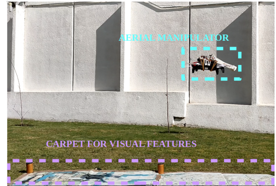
Figure 6: Outdoor scenario. A carpet is set in the ground to provide more texture for the SLAM technique and improve the pose estimation.
