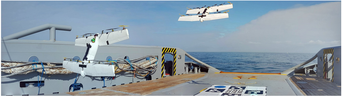
Figure 10: A composite photo from a NederDrone 1 prototype in hover and subsequently in forward flight, operated from a ship on the North Sea.
