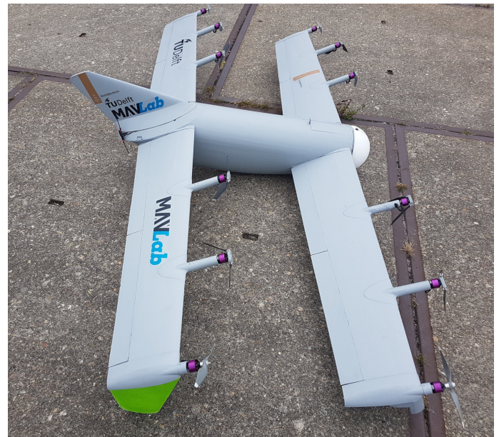
Figure 1: NederDrone2 with 12 propellers of which 8 are fold-able and stop during forward flight. The 4 tip propellers remain active during forward flight and have a higher pitch for efficient fast flight. The large fuselage can accommodate a 9 liter pressure tank and a fuel-cell.
