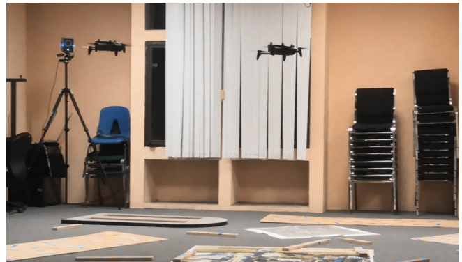
Figure 1: We present a methodology to perform an autonomous coordinate flight indoors using the same controller for both MAVs. We use the onboard monocular camera to metric localisation. A video of this work is found at https://youtu.be/Tcox2MpRGry
