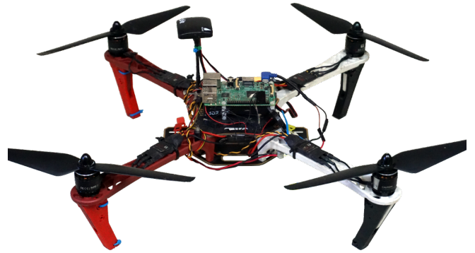
Figure 4: UAV with onboard computer and wifi link used for field experiments
