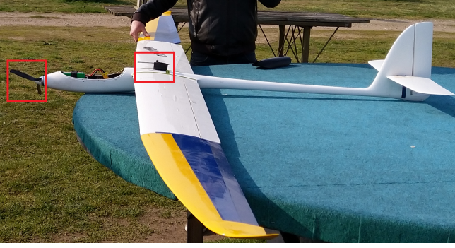
Figure 5: Plane with highlighted propeller and Pitot probe.
