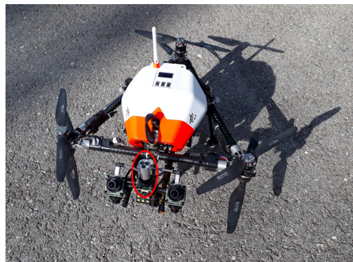
Figure 1: Multicopter “ARDEA” with a frame in triangle shape, three pairs of counter-rotating rotors and a sensor suite mainly consisting of an IMU, two pairs of wide-angle stereo cameras and an insect-inspired polarization compass (highlighted by red ellipse).
