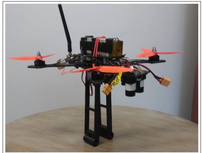
Figure 1: Vehicle used for the Vertical Flight Society's competition with the optical flow (later replaced by RealSense).
