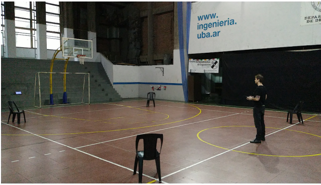
Figure 4: Environment setup for the experiments. The stationary beacons are placed on chairs at a height of 40cm, in a square of 8x8m.
