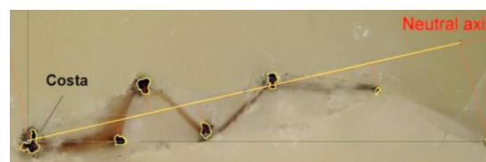
Figure 2 - Cross section through wing of Petalura ingentissima set in wax with corrugation depth \sim 1.1 mm, see acknowledgements
