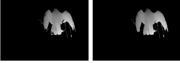
Figure 10: Left image: spatial smoothed disparity map, right image: spatial and temporally smoothed disparity map – gray values from dark gray to white indicate higher disparity and lower depth value – mask is applied to the picture (black background)
