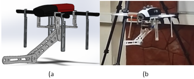
Figure 3: Aerial Manipulation system implemented for this work.
