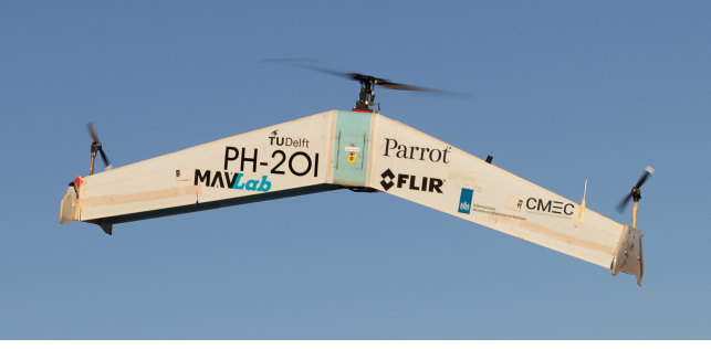
Figure 2: DelftaCopter in hover. In forward flight, the entire fuselage pitches down 90° and the rotor provides the thrust as shown in Figure 1.
