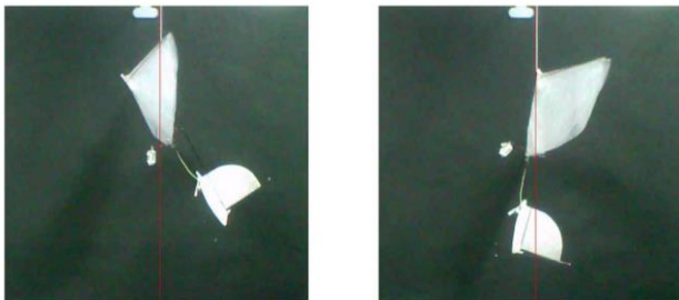
Figure 5 - images of hanging experiments to measure COG
