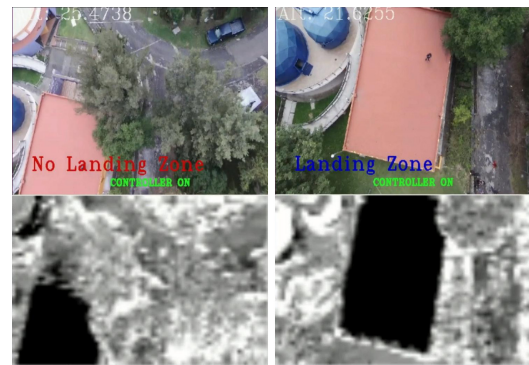
Figure 1: Our proposed system uses two processes, a depth image estimator and a zone classification of single aerial images, aiming at automatically detecting zones that are safe for landing, see video example in: https://youtu.be/E8TZfErP8F8
