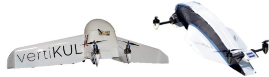
Figure 1: Left: VertiKUL 1, designed to make a transition of 90^\circ with a large wing to provide all the lift. Right: VertiKUL 2, designed to make a transition of 45^\circ with smaller wings to improve wind gust resistance.
