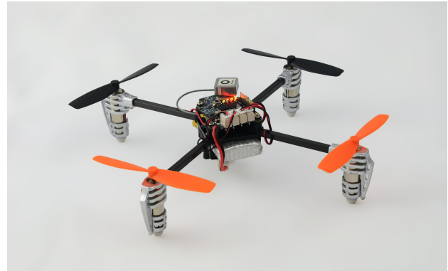
Figure 9: Ladybird 8.5 by 8.5 cm with Lisa-S and the Taoglas Ceramic GPS antenna
