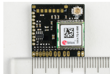
Figure 3: LISA/S V0.1 bottom: showing Ublox GPS module
