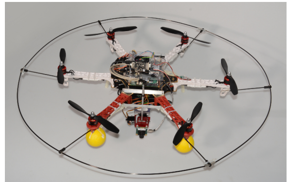
Figure 2: The hexacopter. The diameter of the frame is 62 cm, or 85 cm including the protection ring.
