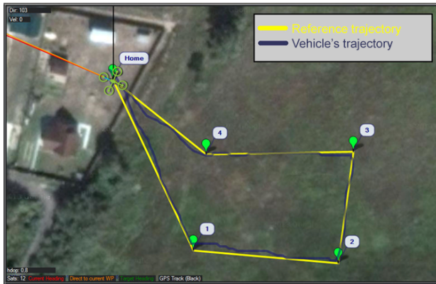
Figure 15: MAV trajectory in waypoint flight
