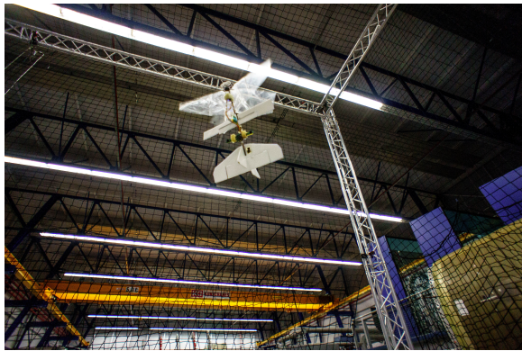
Figure 2: The DelFly in the Cyberzoo; the motion tracking cameras are fixed to the struts shown in the image
