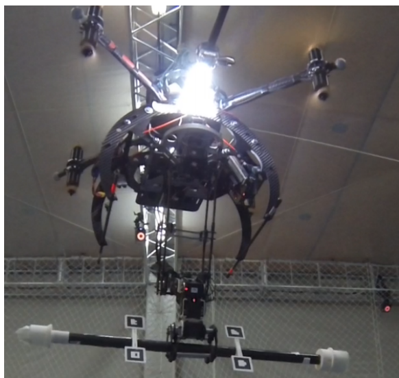
Figure 7: Grabbing a bar with visual markers.
