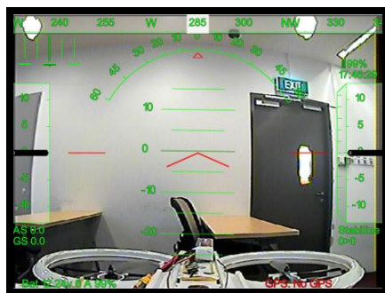
Figure 11: Heads up Display with FPV Camera
