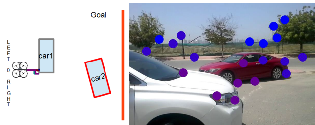
Figure 10: The path of the AR.Drone between two obstacles, without depth classification
