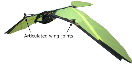
Figure 1: The SlowHawk2 flapping wing flying robot with articulated wings.
