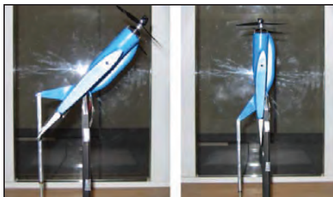
Figure 4: Angle of attack is modified by raising or lowering the rear support
