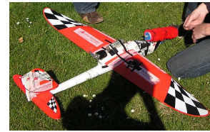
Figure 11: AVS probe mounted on the nose of the MAV
