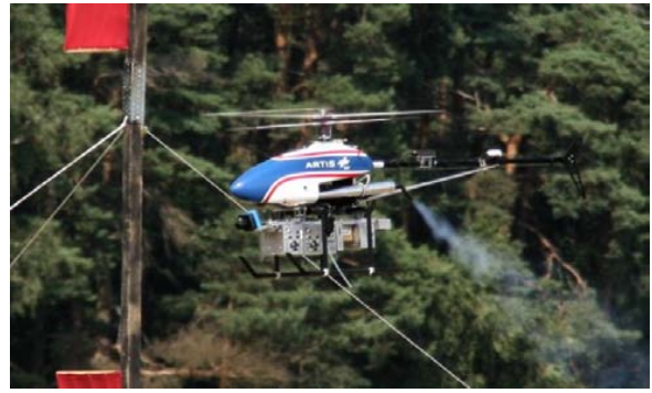
Fig. 2: Research UAV ARTIS: a combustion-engine-powered autonomous helicopter, 1.9m rotor diameter, 12kg gross weight
