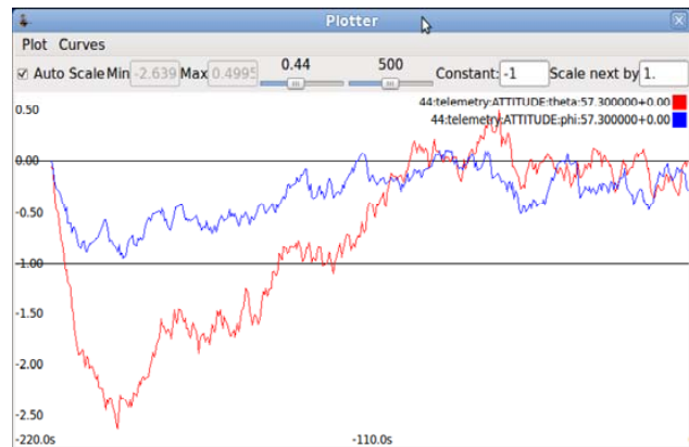
Figure 17: Stabilization of rolls and pitch angel after power up.
