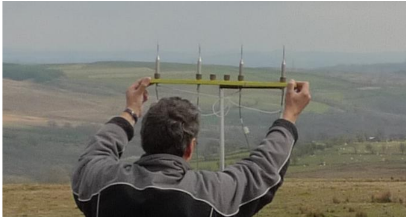
Figure 2 Outdoor Measurements of Atmospheric Turbulence at Four Laterally Separated Points in Space
