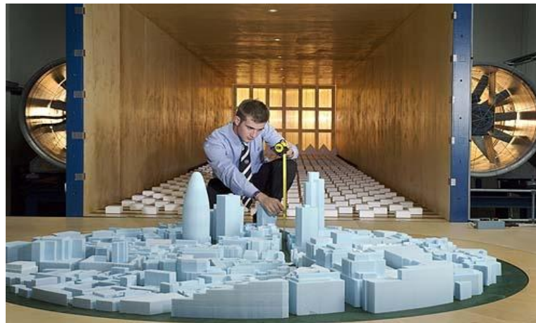
Figure 1 A Typical, Reduced Scale Building Aerodynamics Wind Tunnel Test; Note the Upstream Grid and Roughness Blocks to Generate Turbulence
