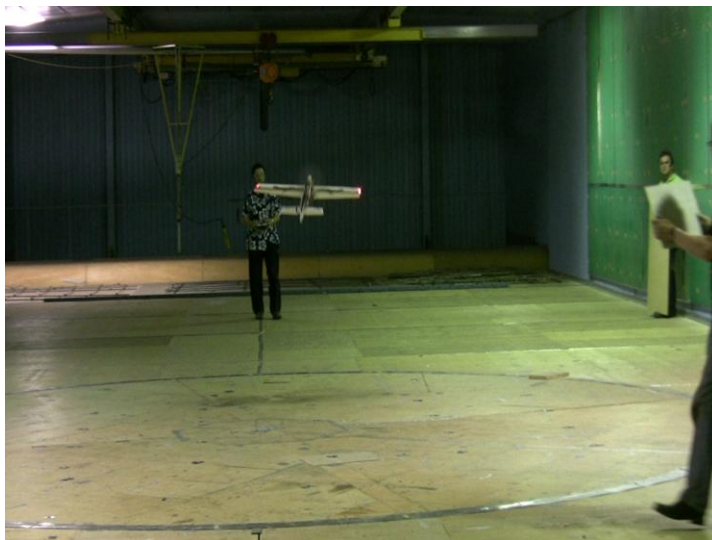
Figure 7 Closed-Loop Flight Into Deeply Stalled Conditions
