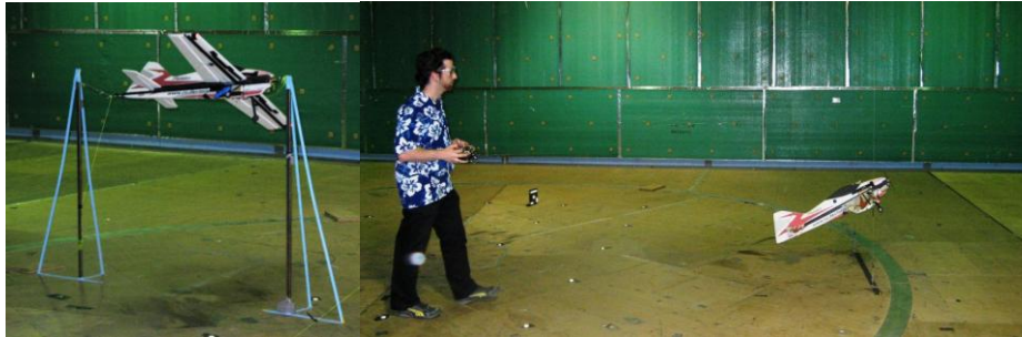
Figure 5 Rigs Used for Isolating a) Roll Inputs, and; b) Pitch and Heave Inputs
