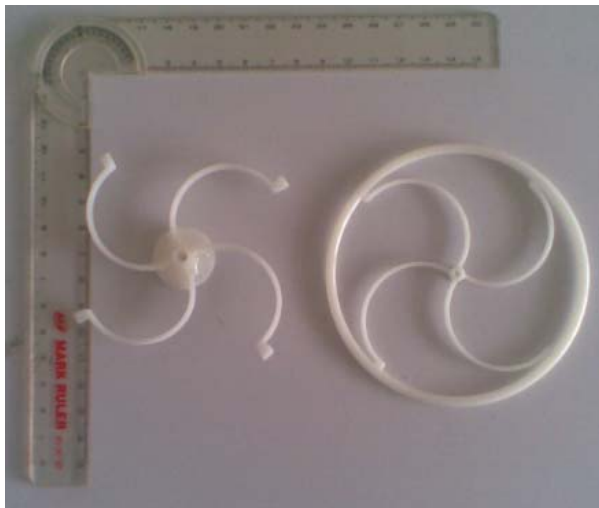
Fig. 8. Left, the "leg". Right, un-modified the light weight wheel. Note: each side of the ruler indicates 15cm.
