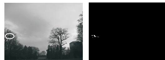
(a) Original image with marked helicopter position (b) Detection result
