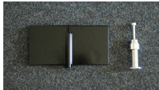
Fig. 5. Flat plate MAV wing with aspect ratio AR=2 and dummy model for flat plate MAV wing with aspect ratio AR=2
