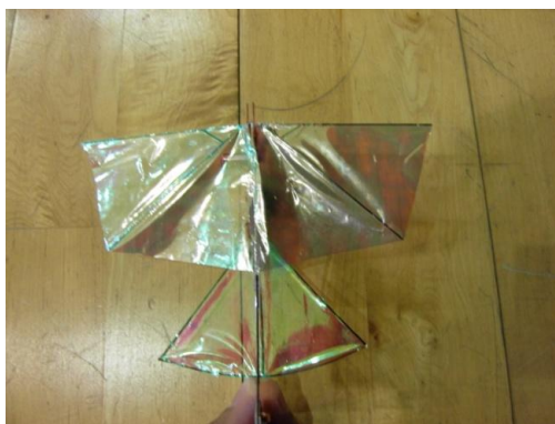
Figure 1: Original 15 cm Flapping-wing Air Vehicle
