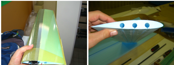
Figure 10: Surface quality and holes for steel rods simulating battery weight and inertia.
