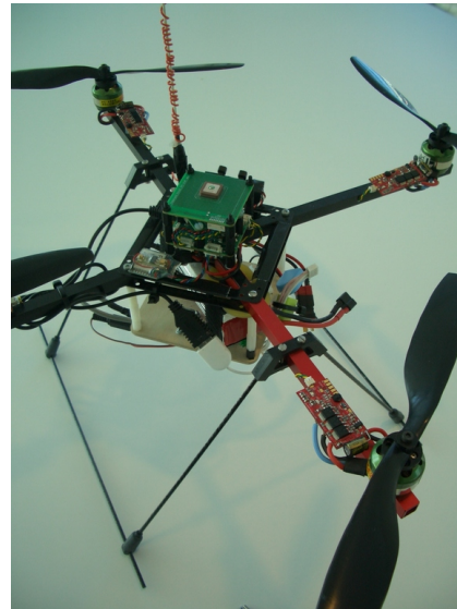
Figure 1: Quadrotor airframe, total flying weight 700 g, typical flight time 15 minutes.
