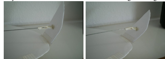
Fig. 20. The deflection of the winglet on the MAV. Note the mechanical linkage.
