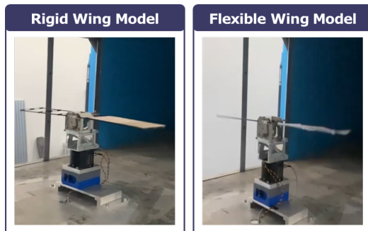
Figure 6: Test model mounted in the KAIST subsonic wind tunnel
