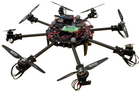
Figure 2: Photo of the canted-rotor planar octorotor UAV
