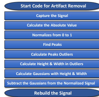
Figure 4: Proposed algorithm for automatic removal of artifacts in real-time.
