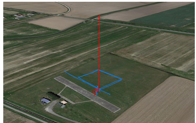
Figure 9: Trajectories for the outdoor flights: vertical profile in red, horizontal square at constant altitude in blue
