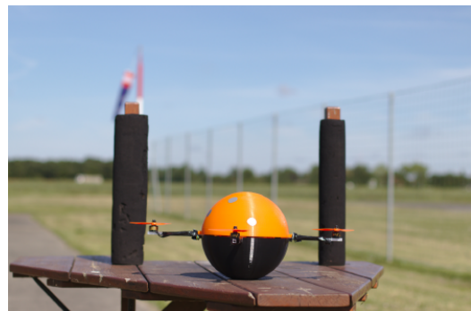
Figure 2: Quadrotor with custom spherical body shape
