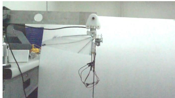
Figure 8: Equipment in force sensor thrust test.
