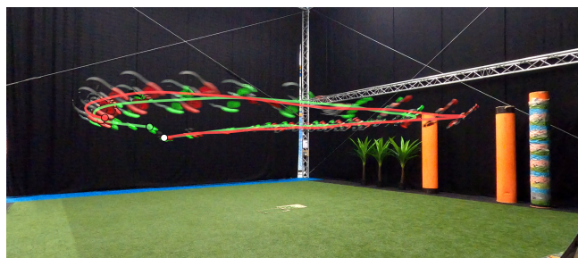
Figure 1: A comparison of a circular flight path between the proposed controller (green) and a classical PID controller (red)
