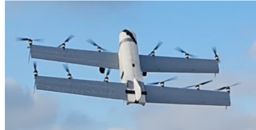
Figure 1: The NederDrone, capable of performing VTOL. The tail-sitter has 20 actuators (12 motors and 8 elevons) and the energy is stored in a hydrogen tank.
