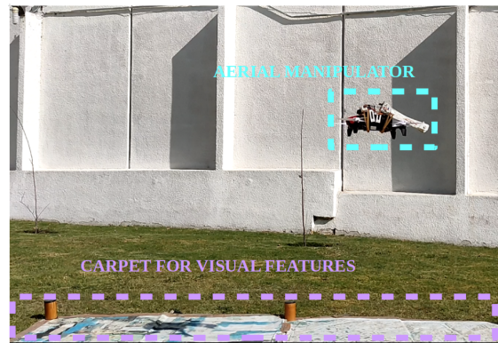
Figure 6: Outdoor scenario. A carpet is set in the ground to provide more texture for the SLAM technique and improve the pose estimation.
