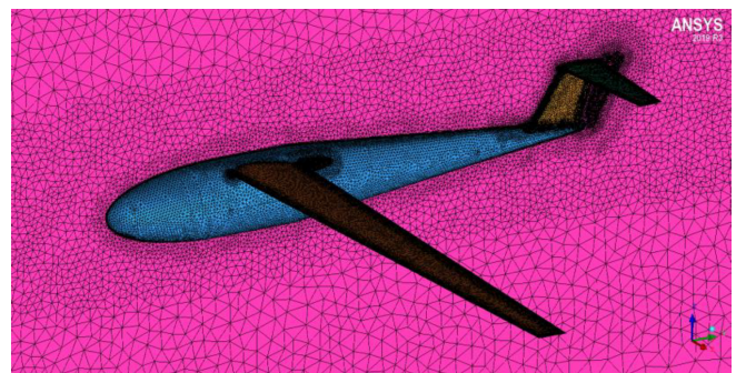
Figure 6: Surface mesh on the first baseline (v1) version of the airplane.
