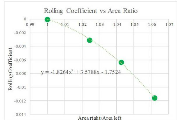
Figure 13: Relationship between rolling coefficient and area ratio.
