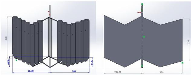
Figure 8: Folding wing level 2 (actual: left, simplified: right).
