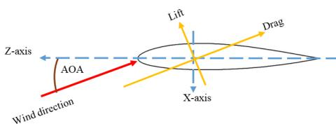
Figure 2: Aircraft axis and aerodynamic force axis.
