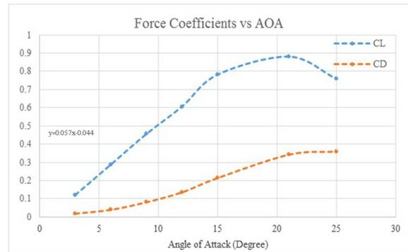
Figure 10: Force coefficient vs angle of attack.
