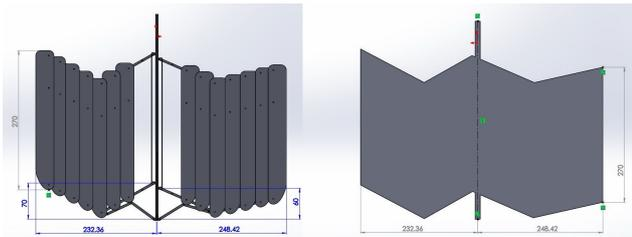
Figure 9: Folding wing level 3 (actual: left, simplified: right).
