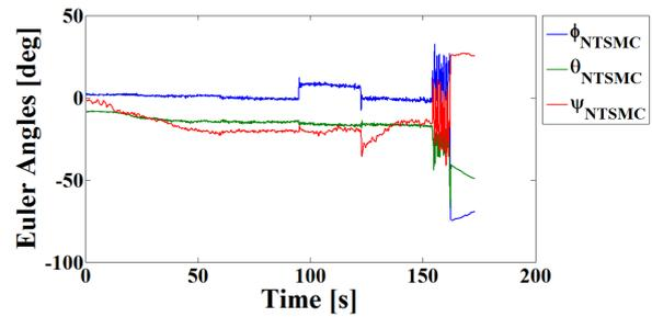
Figure 3: Time history of Euler angles using NTSMC.
