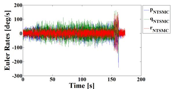
Figure 5: Time history of Euler rates using NTSMC.
