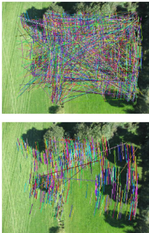
Figure 2: Movement of the matched features from two consecutive frames with unfiltered matches on the top and filtered by ratio test and hamming distance on the bottom.
