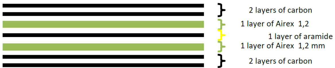
Figure 3: Sandwich composite structure of the arms
