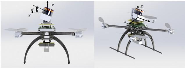
Fig. 2: Rotating angle illustration in front view and isometric view.
