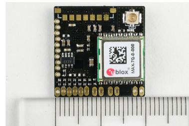
Figure 3: LISA/S V0.1 bottom: showing Ublox GPS module
