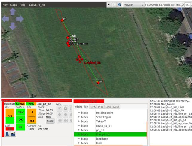
Figure 11: **Paparazzi-UAV** ground station during an autonomous flight of a **Lisa-S** equipped Ladybird
