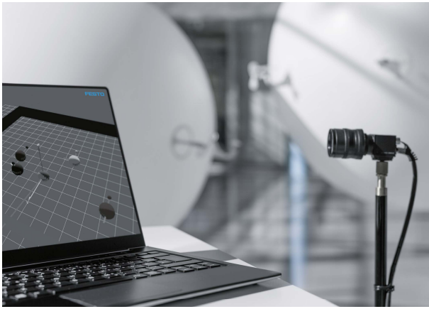
Figure 4: Infrared cameras are used for exact positioning of the spheres.
