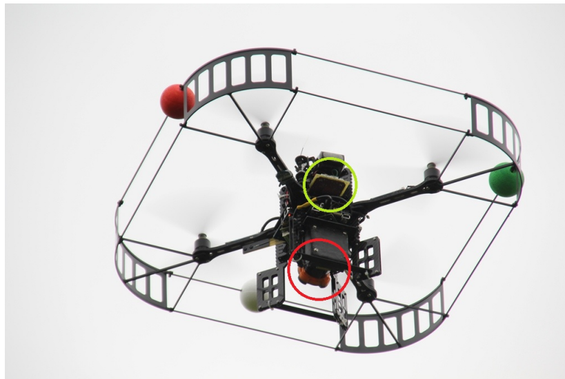
Figure 3: Quadcopter with additional components: laser scanner (red circle), Sensor Readout Unit (green circle)
