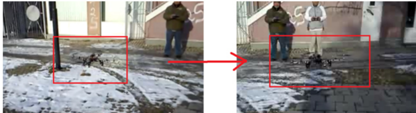
Figure 11: Left: hovering and vector thrust is activated. Right: 2 seconds after activation. Note: the quad moved in Y-axis without any attitude change.
