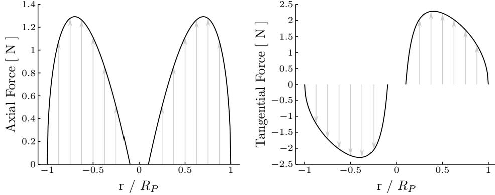
Figure 5: Axial and Tangential Forces for the Modified FINE/Marine Propeller Model
