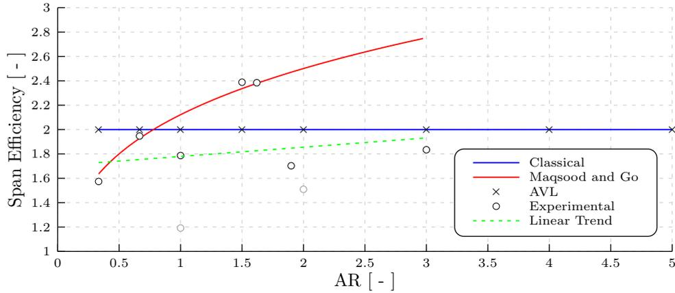
Figure 3: A Comparison of the Theoretical Models for Span Efficiency and Wind Tunnel Experiments. Models from [2, 6, 17], additional experimental data from [3, 6, 17].
