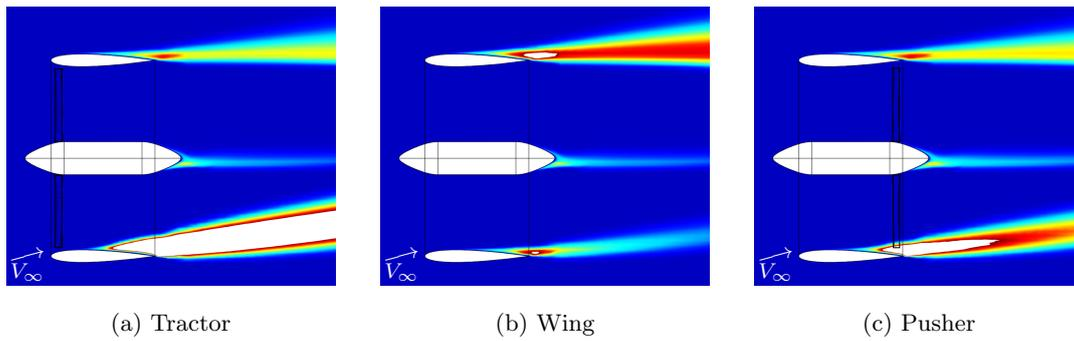
Figure 12: Turbulent Viscosity Showing Differing Stall Characteristics between Each Configuration. Angle of Attack = 15 deg,  $T = 2.5$  N,  $Re = 1.94 \times 10^5$ , scale from blue ( $\mu_t/\mu = 0$ ) to red ( $\mu_t/\mu = 120$ ).
