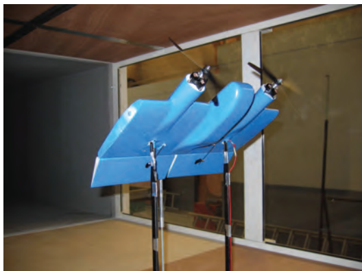
Figure 1: The MAVion, a tandem-rotor tilt-body configuration
