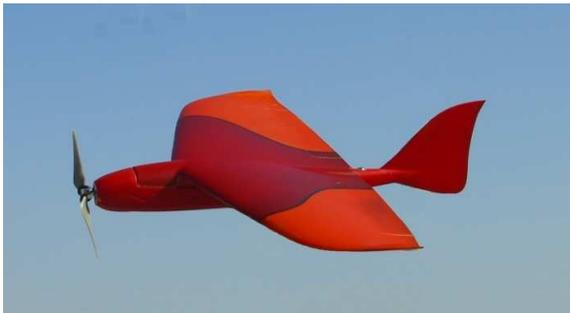
Figure 15: Fire-Storm designed for EMAV09 Endurance mission
