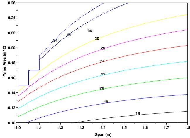
Figure 7: Total weight ( $N$ ) at 20  $m/s$  cruise speed.
