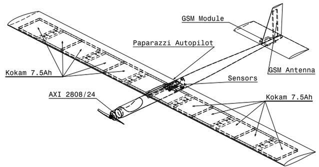
Figure 8: Sketch of the prototype with its components.
