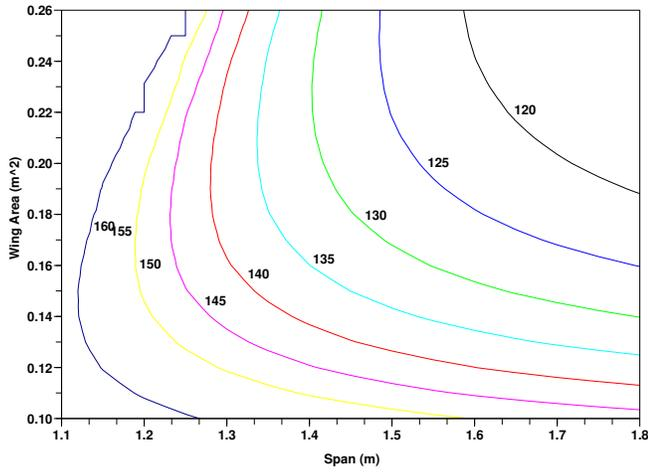
Figure 6: Wing-loading ( $N/m^2$ ) at 20  $m/s$  cruise speed.
