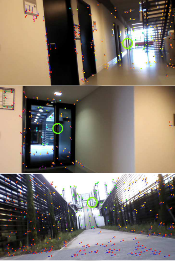
Figure 5: Sparse 3D reconstructions: Blue/purple lines show optical flow vectors consistent/conflicting with the camera’s motion. The points’ color represents their longitudinal distance – red indicates 1 m and below, cyan for 10 m and above. A larger circle marks the target flight direction.
