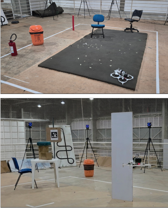
Figure 3: Experimental Setup. (a) Controlled indoor flight volume for the open-vocabulary object-goal trials, with the quadrotor, marked operating bounds, and everyday referents. (b) Cluttered setup for the path-planning trials (Sec. 4.3), with a table, chair, tool case, and a freestanding vertical panel placed between the take-off pose and the trash-bin referent.
